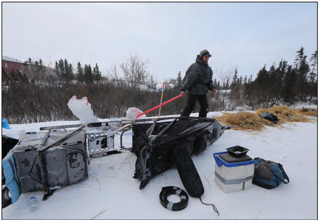
SLED MAINTENANCE — Matt Failor used the break in Koyuk to change his runner plastic. Photo by Diana Haecker
